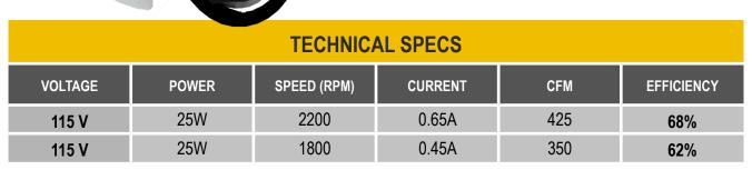
\* Class B insulation supplied for Standard motors but all other insulation classes are also available
