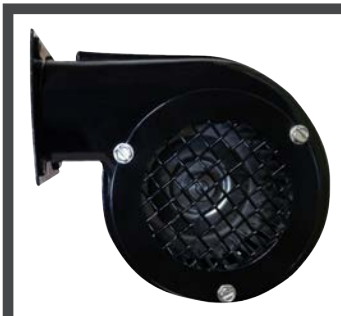
1/40 HP, 115/230V, 0.4/0.2A 50/60 HZ, 3000 RPM, PSC. CRESCOR REF.0769 - 180K, 85CFM MODEL: N1608073
