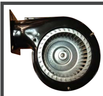
1/35 HP, 115 V, 1.0 A, 50/60 HZ, 3300 RPM, SP, FASCO REF.702112995, 90CFM MODEL: 8211715130
