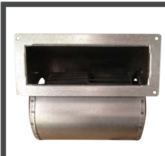
1/8 HP, 208/230V, 1.2A 50/60 HZ, 3250 RPM, PSC EBM-PAPST D2E133-AM47-23, 460 CFM. MODEL: N1601022C
